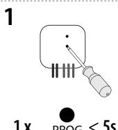
Press of Prog button for 3 - 5s will activate actuator RFDAC-71B into programming mode. LED is flashing in 1s interval.
