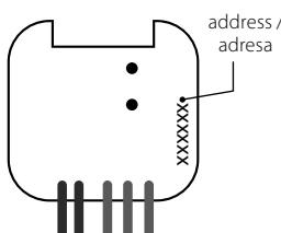
The address listed on the front of the actuator is used for programming and controlling actuators by RF control units.
