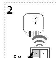
Assignment of the sunrise function is performed by five presses of the selected button on the RF transmitter (must be a lapse of 1s between individual presses).
