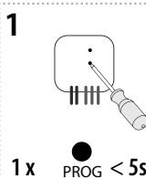
Press of Prog button for 3 - 5s will activate actuator RFDAC-71B into programming mode. LED is flashing in 1s interval.
