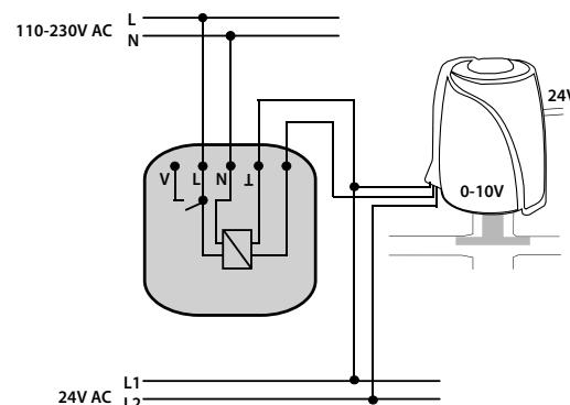
connection with a controlled dimmer (e.g. DIM-6) for dimming up to 2000VA
