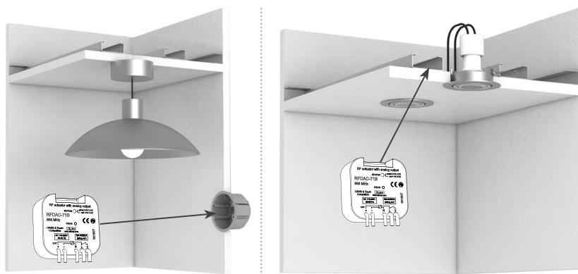
connection with a controlled dimmer (e.g. DIM-6) for dimming up to 2000VA
