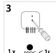
Press of programming button on actuator RFDAC-71B shorter then 1 second will finish programming mode. The LED lights up according to the preset memory function.
