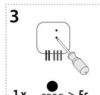
Press of programming button longer then 5 seconds, will activate actuator into timing mode. LED flashes 2x in each 1s interval. After releasing the button, the time of the sunrise function begins to count down (period of complete illumination of the light).
