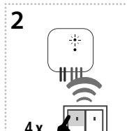
Four presses of your selected button on the RF transmitter assigns the function light scene 4 (must be a lapse of 1s between individual presses).
