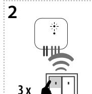
Three presses of your selected button on the RF transmitter assigns the function light scene 3 (must be a lapse of 1s between individual presses).
