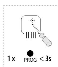
Selecting the output voltage mode 0-10V or 1-10V is performed by pressing the PROG button for 1 - 3s.
