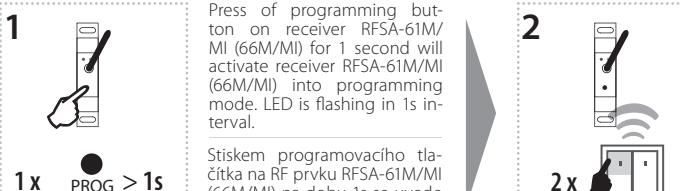
Two presses of your selected button on the RF transmitter assigns the function switch on (must be a lapse of 1s between individual presses).
