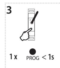
Press of programming button on receiver RFSA-61M/MI (66M/MI) shorter than 1 second will finish programming mode. The LED lights up according to the pre-set memory function.
