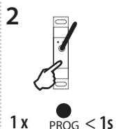
Pressing the programming button on the RFSA-61M/MI (66M/MI) receiver for less than 1 second will finish the programming mode, this will reverse the memory function. The LED lights up according to the current pre-set memory function. The set memory function is saved.
