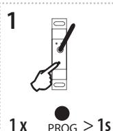
Press of programming button on receiver RFSA-61M/MI (66M/MI) for 1 second will activate receiver RFSA-61M/MI (66M/MI) into programming mode. LED is flashing in 1s interval.
