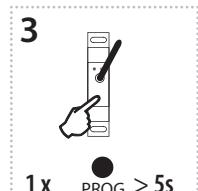
Press of programming button longer than 5 seconds, will activate actuator into timing mode. LED flashes 2x in each 1s interval. Upon releasing the button, the delayed return time starts counting.
