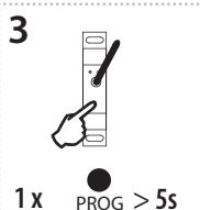
Press of programming button longer than 5 seconds, will activate actuator into timing mode. LED flashes 2x in each 1s interval. Upon releasing the button, the delayed return time starts counting.
