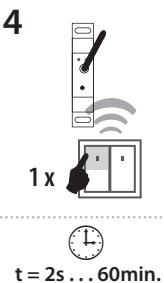
After the desired time has elapsed (range of 2s...60min), the timing mode ends by pressing the button on the RF transmitter, to which the delayed return function is assigned. This stores the set time interval into the actuator memory.
