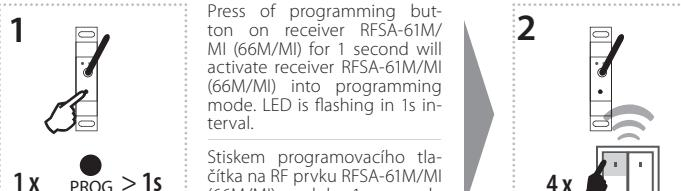
Four presses of your selected button on the RF transmitter assigns the function impulse relay (must be a lapse of 1s between individual presses).
