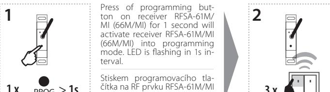
Three presses of your selected button on the RF transmitter assigns the function switch off (must be a lapse of 1s between individual presses).
