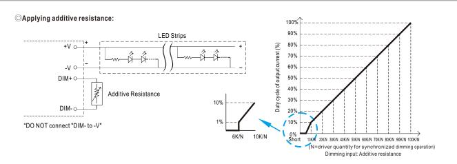
Note: 1. Min. duty cycle of output current is about 1%, and the dimming input is about  $6K\Omega$  or 0.6VDC, or 10V PWM signal with 6% duty cycle. 2. The duty cycle of output current could drop down to 0% when dimming input is less than  $6K\Omega$  or less than 0.6VDC, or 10V PWM signal with duty cycle less than 6%.
